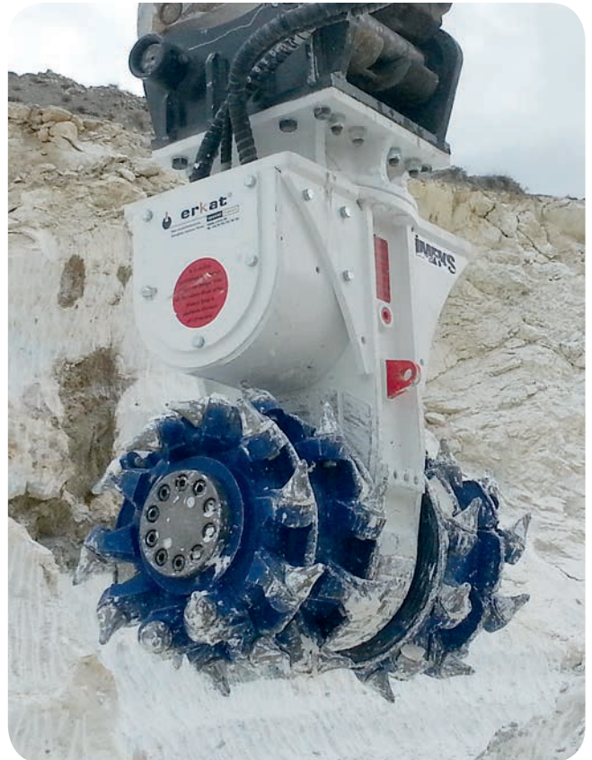
An ER transverse drum cutter cutting rock
